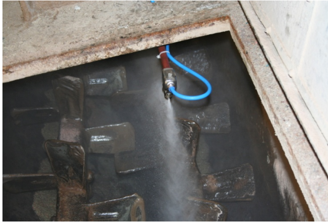
Ideal spray nozzle for application onto granular fertilizer in a blender
