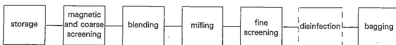
Fig 1. Flowsheet of production process for organic fertilizer.
