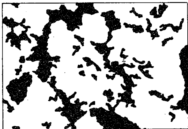
FIG 1 The pore system of a thin slice of uncompressed soil. The dark area represents the voids (Trowse, 1971b).
